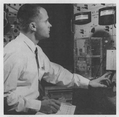
SUBJECTING CAPACITORS to rigorous leakage current and resistance tests is Art Cannon (5523-3) who determines their ability
